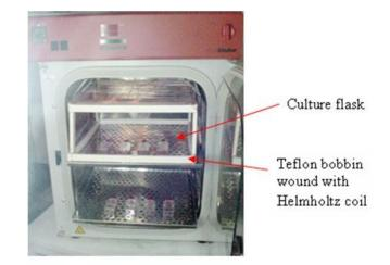
**Figure 7.** Magnetic field exposure facility fabricated using Teflon frame wound with Helmholtz coil housed inside the  $CO_2$  incubator for studies on cellular models.
